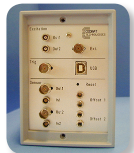
Lamb wave drive and sensing electronic LWDS45. Courtesy FP6 AISHA project.
