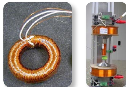
Torus and Permeameter methods.
