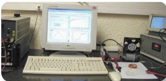
Set-up for measuring magnetic characterization.
