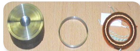
Preparation of raw material UGITECH 416, machining in the form of torus and winding.
