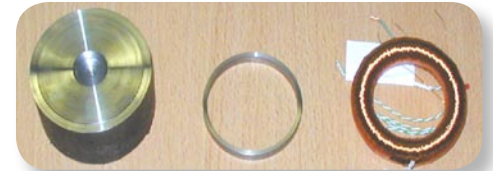
Preparation of raw material UGITECH 416, machining in the form of torus and winding.
