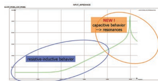
Figure 3: Curve of the impedance Z(f) showing system resonance.
