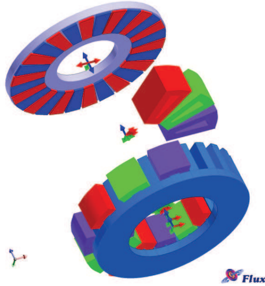
Fig. 3. Three-dimensional FEM model of AFPM
