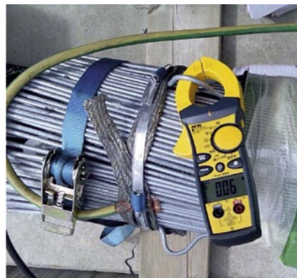
Figure 3. Measured current in armour wires at 90° displaced locations: not possible to distinguish any armour wire current (left: 0,06 A reading) from background interference (right: 0,05 A).
