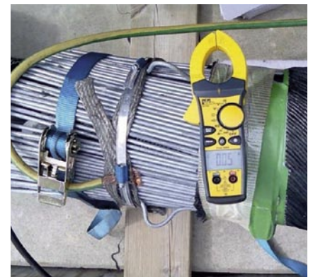
Figure 3. Measured current in armour wires at 90° displaced locations: not possible to distinguish any armour wire current (left: 0,06 A reading) from background interference (right: 0,05 A).
