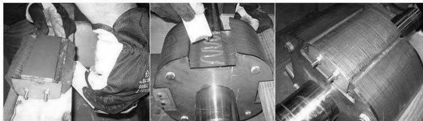
Fig. 2. Manufacturing rotor with dovetail design. In the left there is a pole with magnets, in the middle there is the rotor without the pole, and in the right the pole is inserted to rotor.
