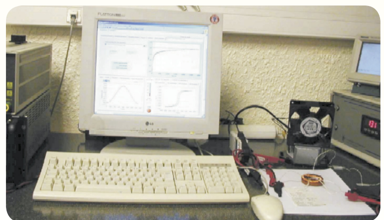
Figure 8: Set-up for measuring magnetic characterization with Laboratorio Eletrofisico gaussmeter.
