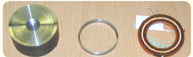
Figure 5: Preparation of raw material UGITECH 416, machining in the form of torus and winding.
