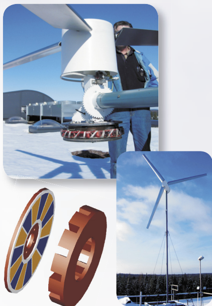
Figure 1. Experimental wind power plant and the used single sided axial flux permanent magnet generator.
