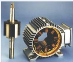
Figure 1: SRM and its drive modelled with FLUX to SIMULINK Technology (courtesy of HWV, Belgium).
