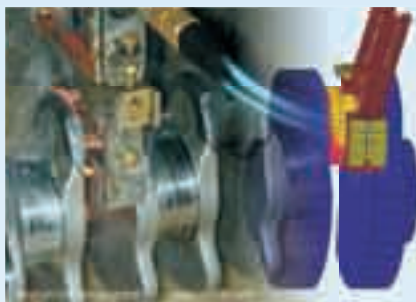
Figure 3: Induction hardening of a crankshaft. Volume density of induced power. Acknowledgments: Prismeca, www.prismeca.fr
