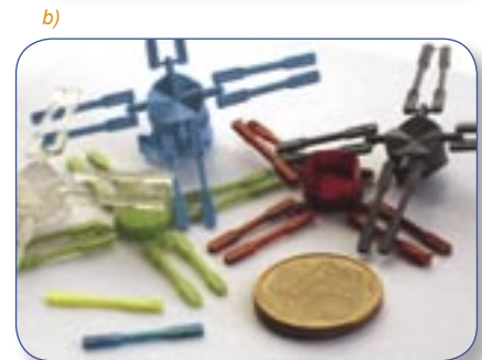
a) - b) : Example of achievement: miniature parts manufactured using ultrasound moulding.
