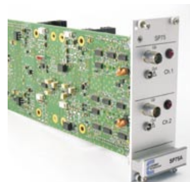
Figure 6.9: View of the SP75A-1 switching power
